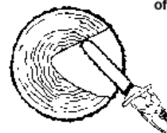
Top or blade nose touches bottom or side of kerf during reinsertion
