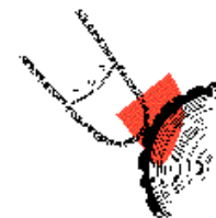
Improper starting of bore
